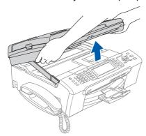
Insert the network cable into the LAN socket marked with a R symbol. You will find the LAN socket inside the machine on the left as shown below.
